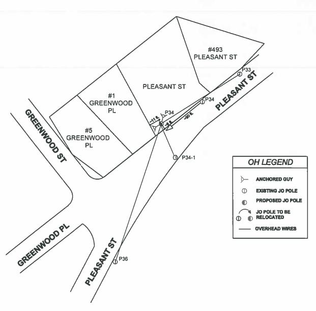
Sketch to accompany an easement for Pleasant Street property for the installation of relocated pole 34 aproximately 6 ft. on to private property along with the installation of associated anchors and overhead wires.
